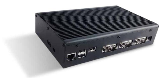
Professional Digital Signage Terminal is an advanced easy signage player where it is powered by embedded Linux OS. User can easily control the signage box by TCP/IP socket communication or serial communication.
